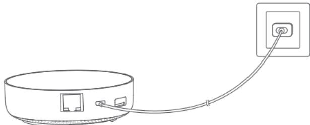
\* If you need to use wired network communication between the hub and the router, please use a network cable with RJ45 network port to connect the LAN ports of the hub and your router, and wait for the orange and green lights on the side of the network port to light up.
